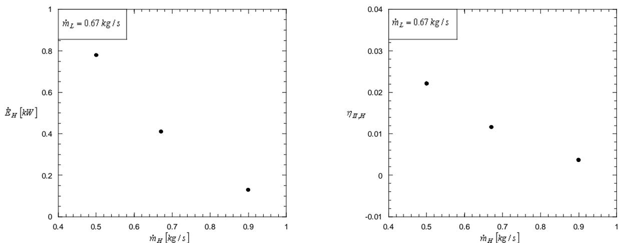
Figure 7. Variations of the hot water flow rate in function of the heating capacity and efficiency.
