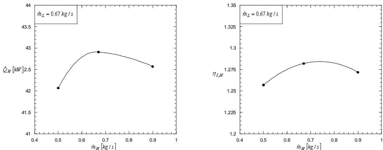
Figure 6. Variations of the hot water flow rate in function of the heating capacity and efficiency.
